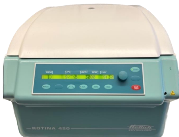
Figure 2.10 – ROTINA 420 centrifuge
