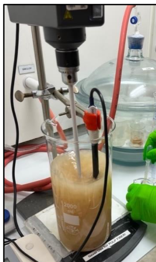
Figure 2.3 – TEMPO-mediated oxidation with pH monitoring
