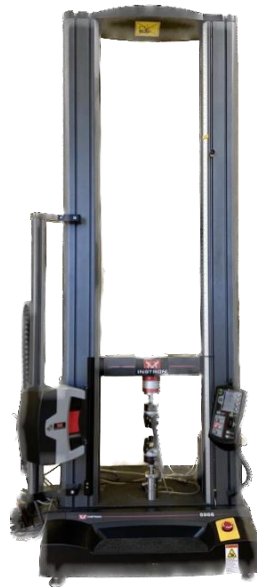
Figure 3.3 – Instron 5966 dynamometer
