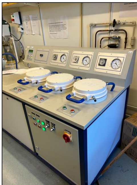
Figure 2.12 – Sheet Former Rapid-Köthen (RL-ASF-A)
