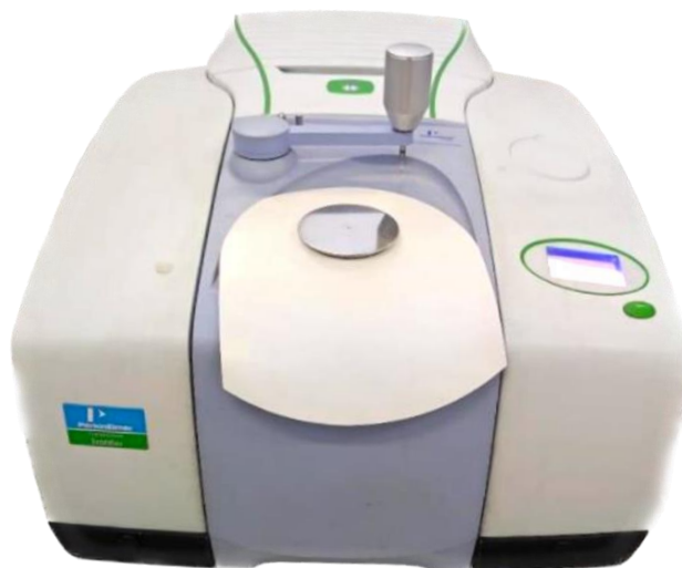
Figure 3.2 – FTIR Spectrometer Frontier in ATR mode
