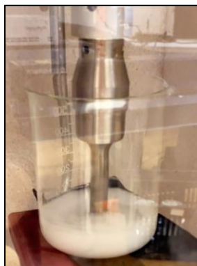
Figure 2.9 – Sonication of h-BN and CNF solutions
