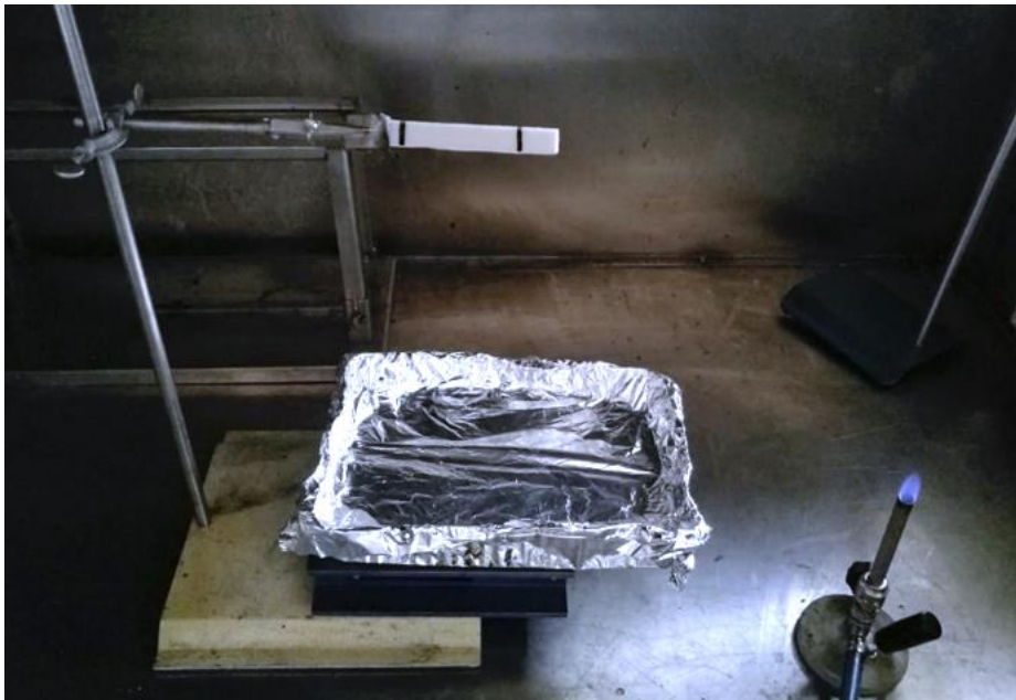
Figure 3.4 – Experimental setup of UL-94 flammability test
