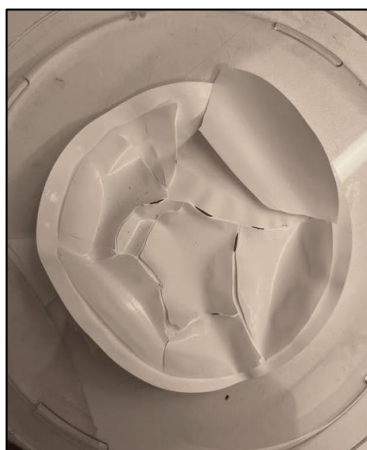
Figure 2.13 –BN/CNF 80% broken dry sample
