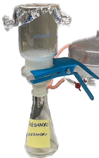
Figure 2.11 –Vacuum filtration with fritted glass setup
